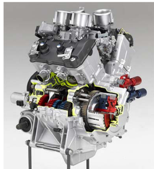
Fig. 1. External view of V4 engine with newly developed Dual Clutch Transmission
